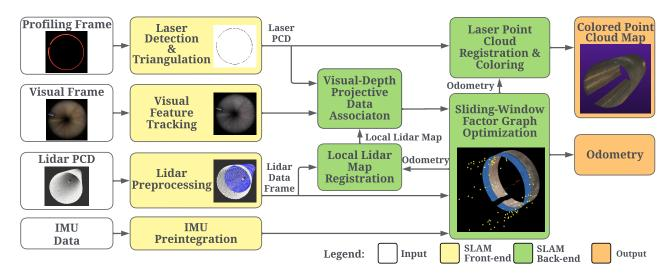
Fig. 3. VILL-SLAM software architecture and information flow chart.
