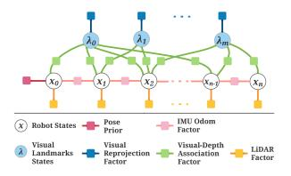
Fig. 4. At the core of our method, a factor graph is used to represent various states with their related constraints within a sliding window.
