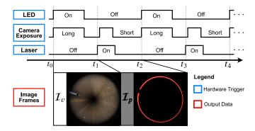
Fig. 2. We capture visual and profiling image frames using one camera by quickly switching between visual and profiling frames using a microcontroller, measuring RGB and depth information in a near-concurrent fashion.
