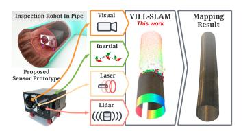
Fig. 1. The in-pipe mapping sensor hardware prototype using the proposed VILL-SLAM method to fuse multiple sensory information, which produces a photo-realistic dense RGB-D reconstruction of a 12-inch pipe segment.
